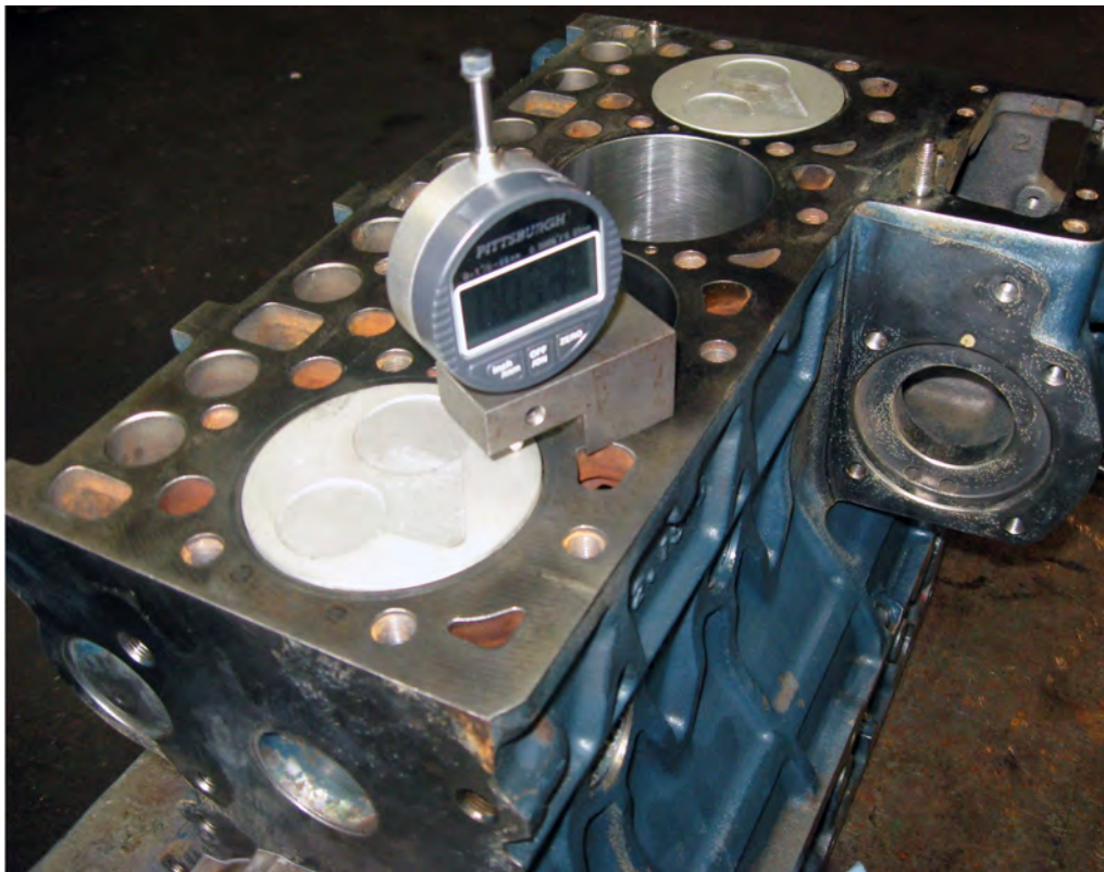
Piston protrusion is checked to install correct head gasket.
