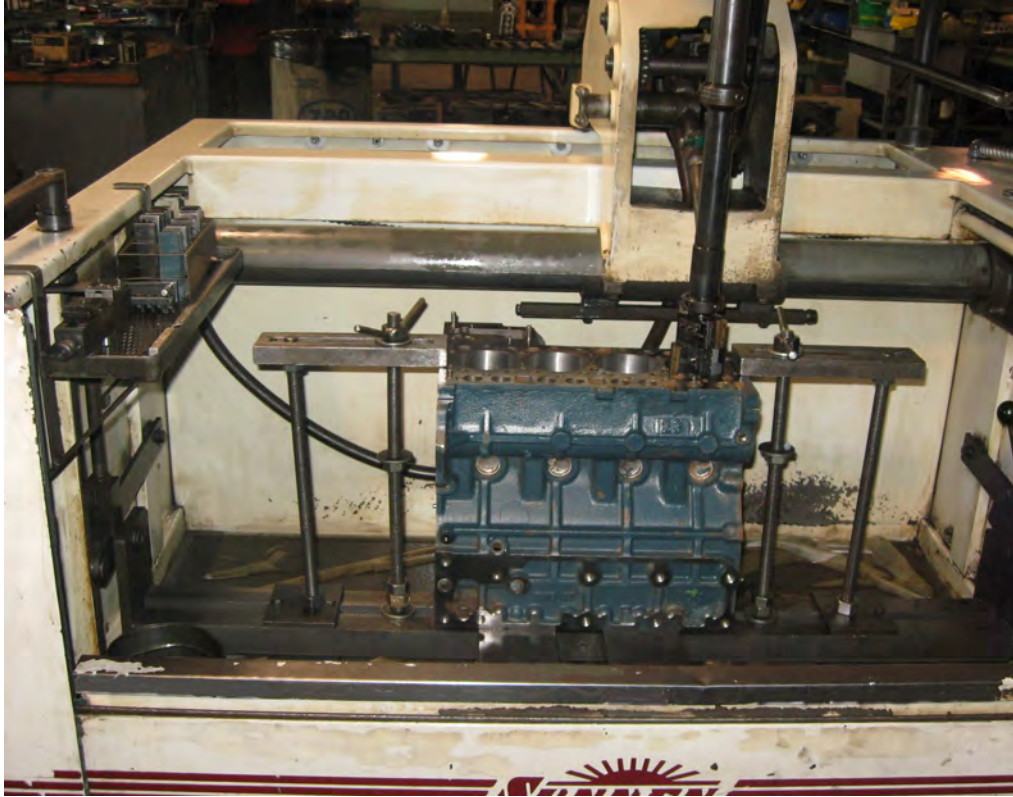
Cylinders are bored and honed to correct size and RA finished for quick ring seating.
